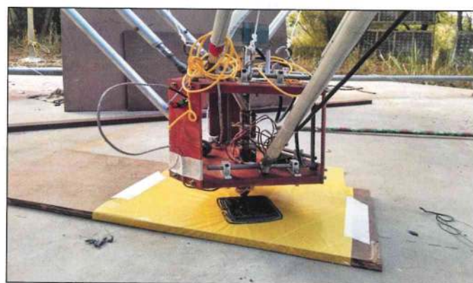
Precision building in three dimensions – the printer in action
